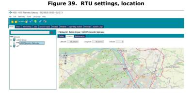
On this tab you can configure settings for the location of the RTU. You can adjust the position via GPS or by positioning it on the map.
