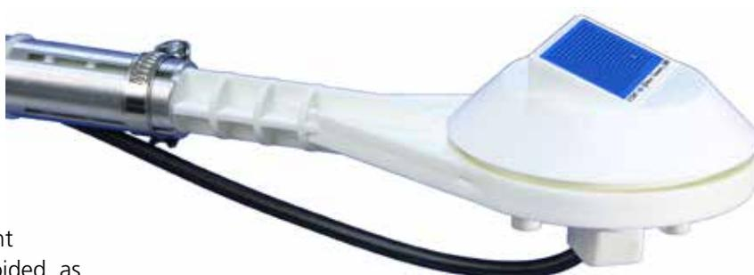
In order to properly simulate the behavior of a leaf the sensor should be installed right inside the foliage. Direct sunlight and excessive exposure to wind should be avoided, as both will significantly shorten the indicated leaf wetness duration.
