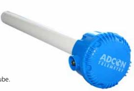
Depending on the length of the sensor up to 5 temperature sensors are available. The 30, 60, 90, 120 and 150cm probes have their first temperature sensor located at 15cm and every additional sensor with a spacing of 30cm, thus at 45, 75, 105 and 135cm respectively.
