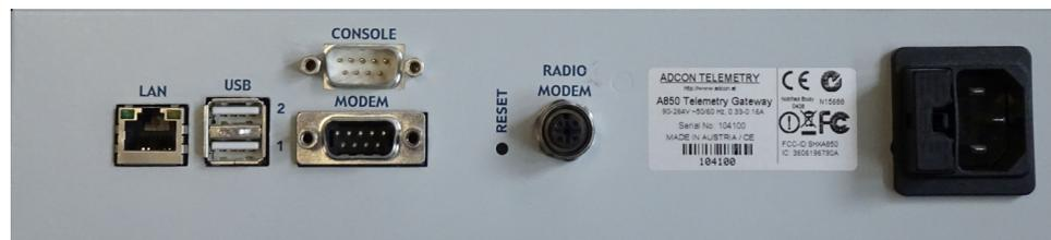
**Figure 4. Back panel of A850-2020 Telemetry Gateway**
