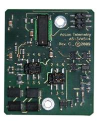
The ADCON A514 Modbus Interface is an adapter than can be integrated into the following Series 4 RTUs:
