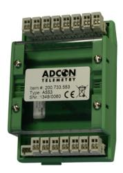
The ADCON A553 was built for industrial applications, which require lots and lots of digital in- and outputs, to monitor equipment, and to switch devices on and off. Each A553 adds 7 digital inputs and 7 digital outputs to a Series 4 RTU. It communicates via the digital pin on each 7-pin connector of an RTU. One such device can be connected per Port. Up to 4 devices can be connected to an A753 RTU, adding 52 digital ports, while one can be added to the A723.
