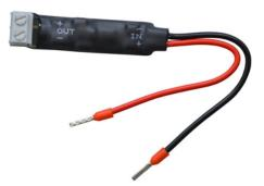
Many sensors, such as the OTT level sensors RLS and PLS, require supply voltages beyond the range an ADCON RTU can supply (5,6 - 7,5V). To enable customers to nonethelss connect these sensors we have developed this inexpensive, yet very efficient step-up converter. It can easily be integrated e.g. inside the top sensor cap of an RLS radar sensor, or inside the FAD box of an OTT PLS sensor.
