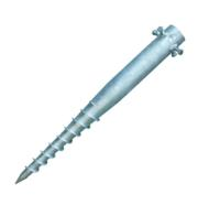
In many cases it is not sufficient to simply pound a pole into the ground. Especially soft soils don't offer enough support to the weight of a weather station. In these cases this soil anchor is a solid alternative. It can simply be screwed into the soil, and, by compatcing the soil around it, will provide a sturdy support to your weather station or RTU mast.
